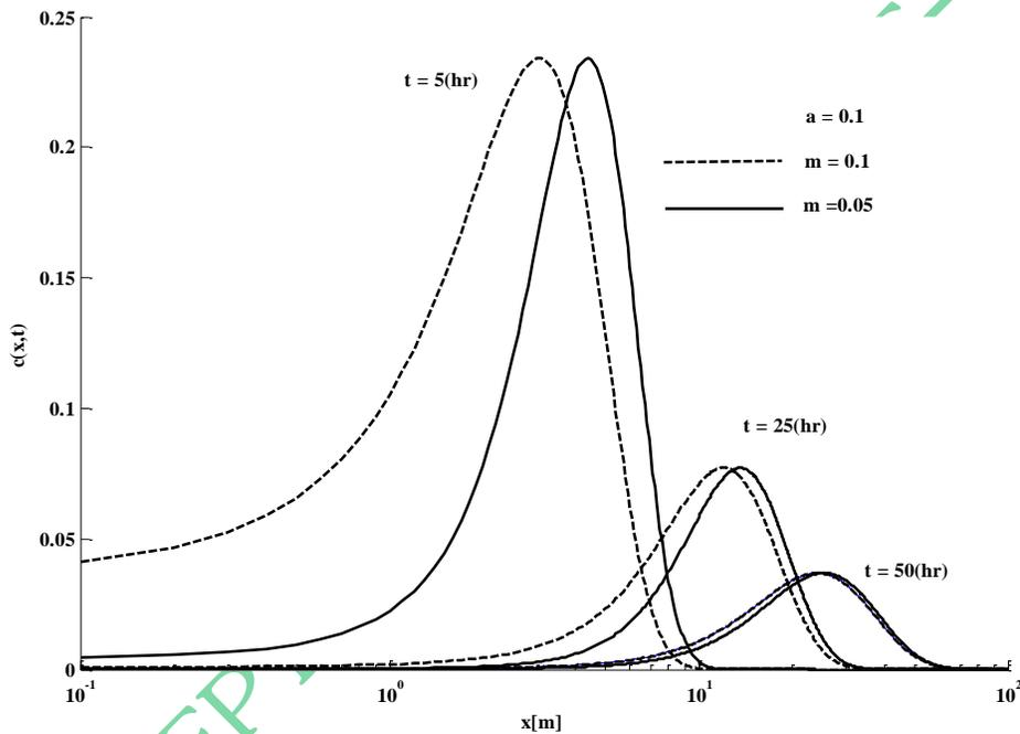
Fig.1. Concentration distribution from instantaneous injection source along heterogeneous medium.
