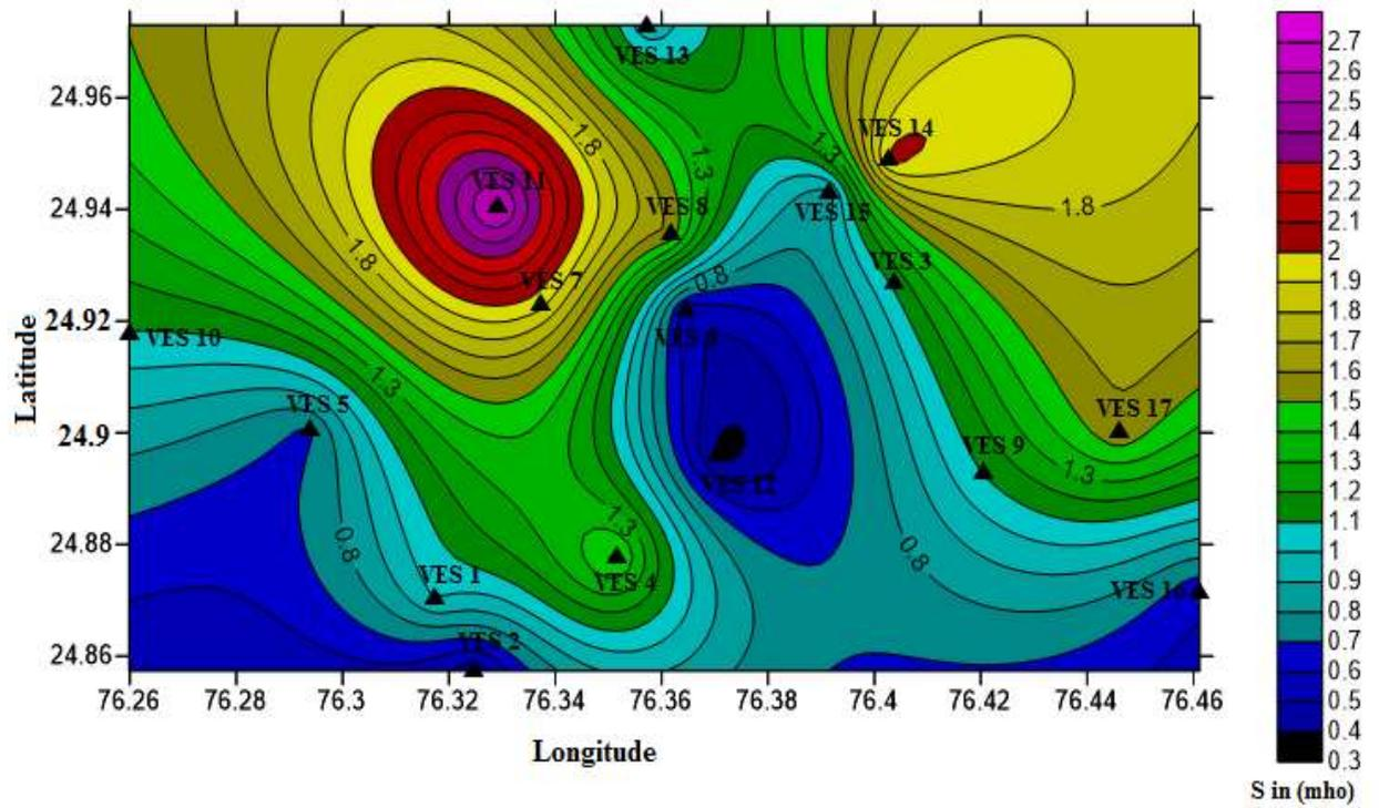
Fig.3. Total longitudinal conductance contour map of the area.
