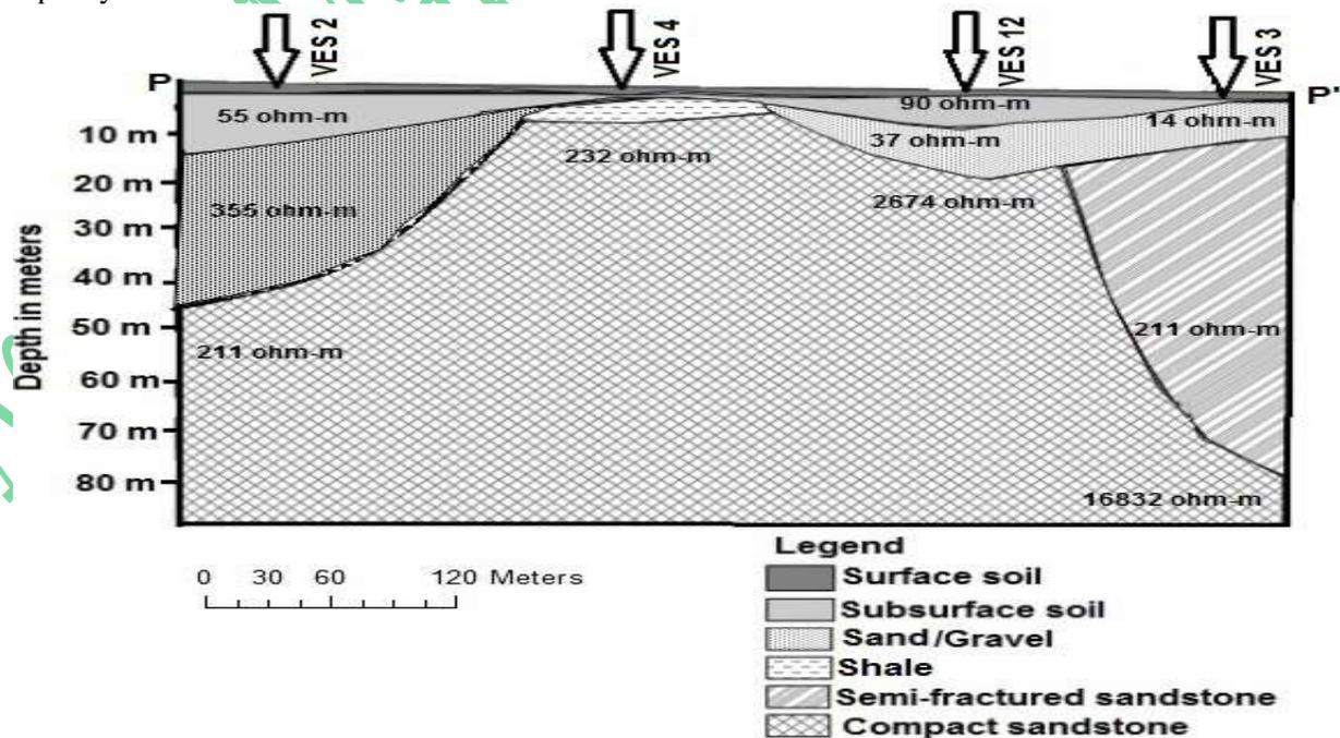
Fig.8. Geo-electrical cross-section along profile PP'.
