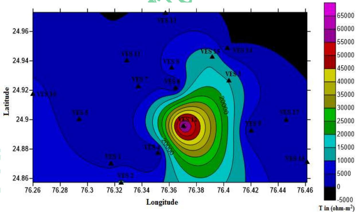
Fig.5. Total transverse resistance contour map of the area.
