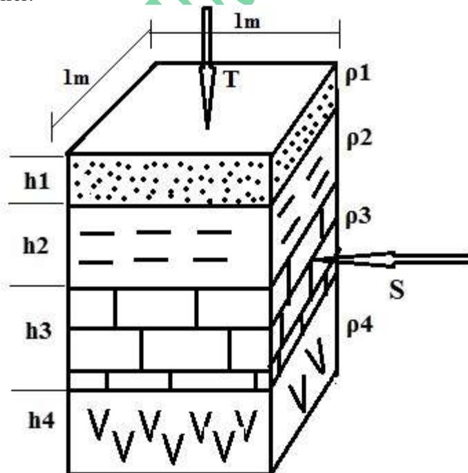
Fig.2. Layered model showing transverse resistance ( $T$ ) and longitudinal conductance ( $S$ ).
