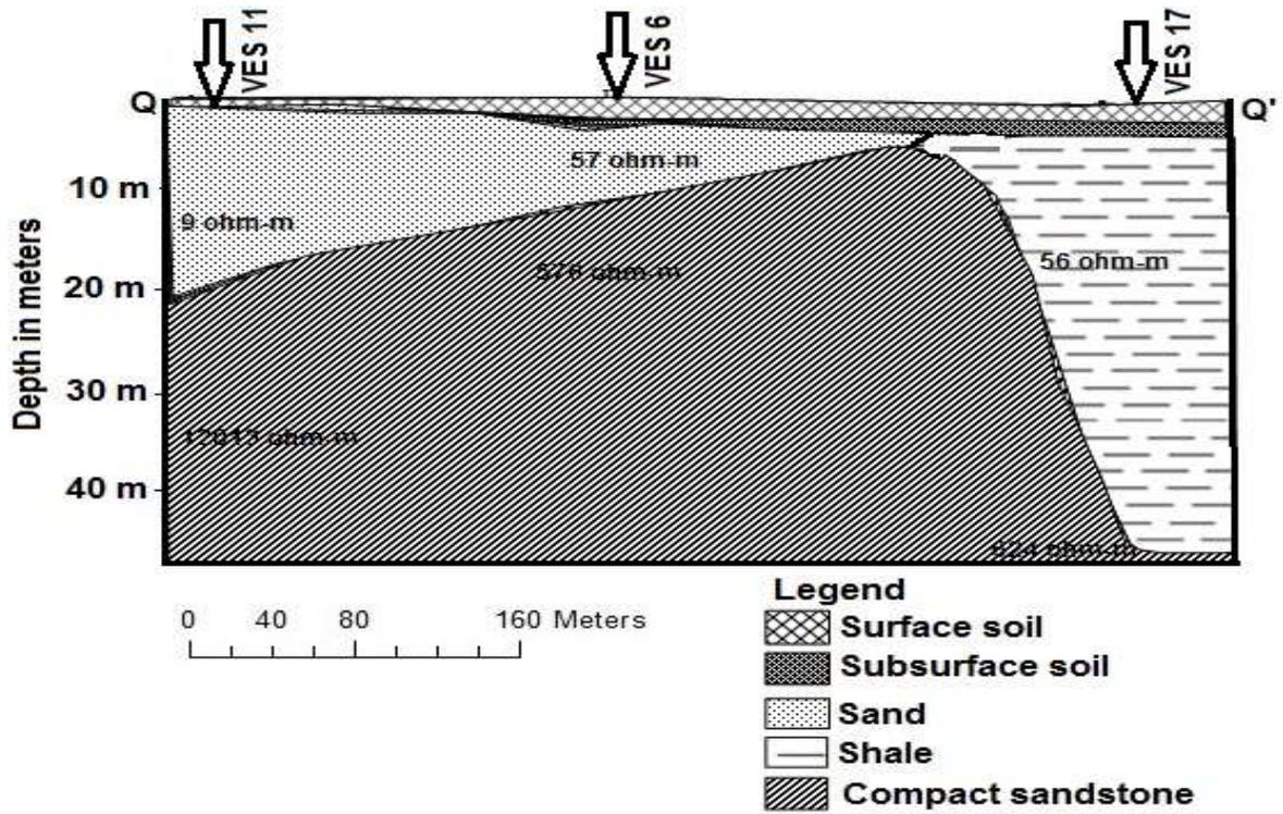
Fig.9. Geo-electrical cross-section along profile QQ'.
